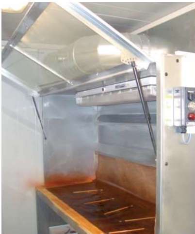
Hazardous materials work station with exhaust technology directing an air stream toward the suction strip on the rear wall. With approx. 0.5 m/s ventilation speed at the 400mm-high intake with the front pane closed.
