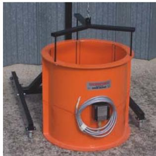
Before lifting, attach the winch hook onto the lifting bar eye. Ensure that the lifting bar is securely attached to the Thermosafe by inserting the 3 spring clips into the closest holes to the underside rim of the heater.
